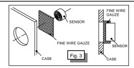
Close the housing as watertight as possible f.i. by using silicone.
