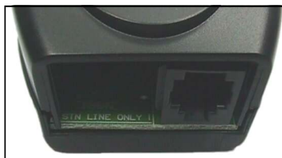
Accepts standard telephone plug
