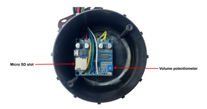
When there is a micro SD card inserted onto the internal module, the micro SD card will replace the built-in flash and will be directly detected as a USB flash drive on computer through plugging into the USB data cable. The device supports max. 32GB micro SD card, so please use a micro SD card within 32GB capacity. Format in FAT32 for the micro SD card is preferable.
