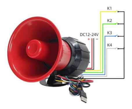
Note: there is an additional black wire (GND) working as COM. It's also possible to directly trigger the horn through a PLC/industrial controller that gives low signal. When it works with a PLC/industrial controller, ground needs to be shared in advance.
