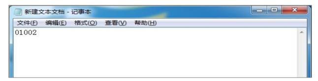
1). As you can see there are 5 digits in the configuration file (it's a text document). The first digit "0" represents the trigger mode of the button (it's purposed for other products), the second and third digits "10" represent the volume setting, and the fourth and fifth digits "02" are the device address.
