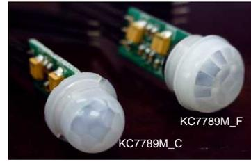
KC7789M is small size PIR sensor module with built-in amplifier and logic circuit. The heart of the module is high reliable PIR controller KC778B. The PIR sensor can be manufacturer specified. The detection angle and distance dependence on the lens used.
